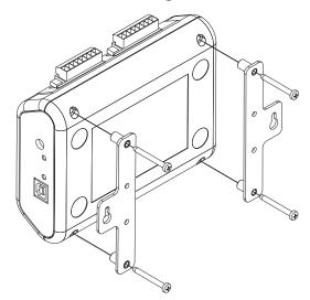
Figure 3-6. OM-DAQ-USB-2401 Wall Mounting
